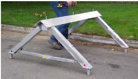
Lock cross braces
