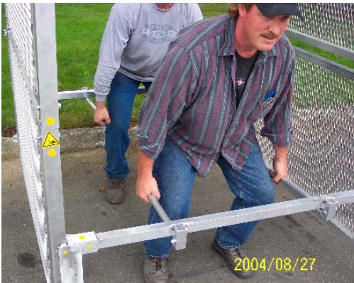
The handles should bend towards the center of the cage for carrying.
