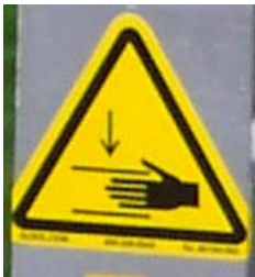
WARNING: Pinch point
