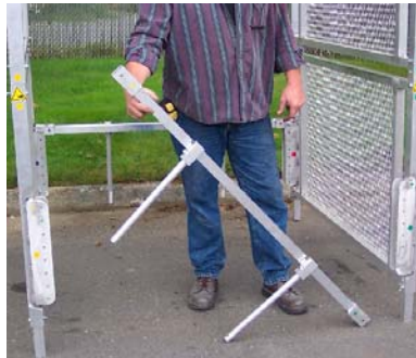
Connect the combo safety bar and lifting handles..
