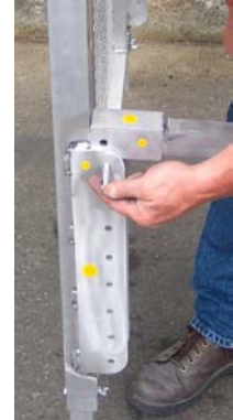
Insert bolts to each side.
